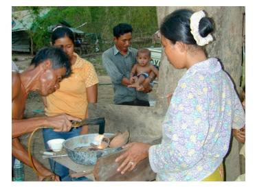
Figure 6. Miner separating mercury from gold (T. Murphy).
