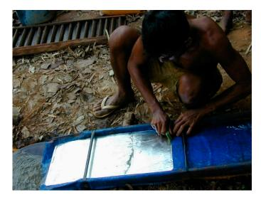
Figure 5. Scraping mercury with gold from flume. (T. Murphy).
