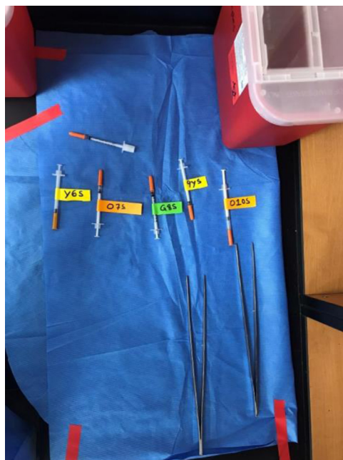
Fig. 1. Extra-long forceps were used to handle the tagged syringes.
