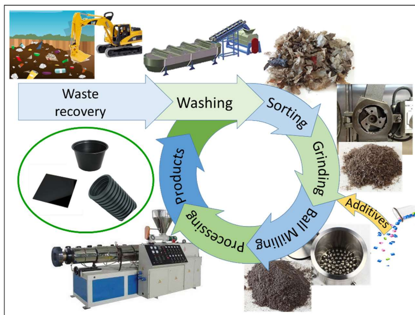
Figure 1. Scheme of the grinding, preprocessing, and processing steps applied to the landfill-recovered plastic (LRP) material.
