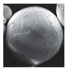
**Fig. 5.** Scanning electron micrograph of microspheres (X1000) having drug to polymer concentration 1:4
