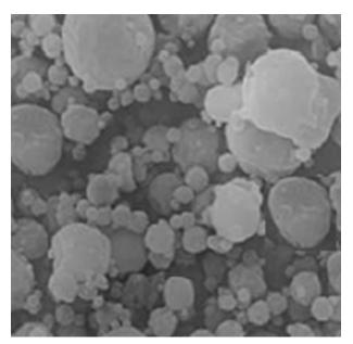
**Fig. 4.** Scanning electron micrograph of microspheres (X100) having drug to polymer concentration 1:1
