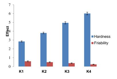
Fig. 7. Effect of locust bean concentration on tablet hardness and friability.
