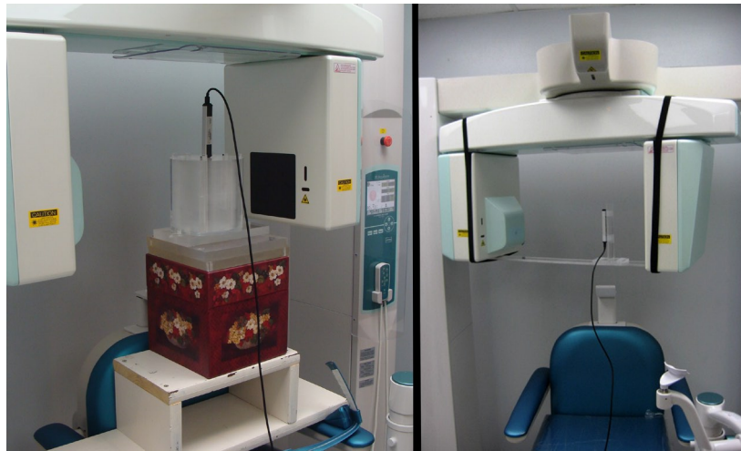
FIG. 3. Setup for measuring HVL at isocenter for the Morita 3D Accuitomo cone-beam CT unit using an Unfors dosimeter (right), and CTDI on same cone-beam unit (left).
