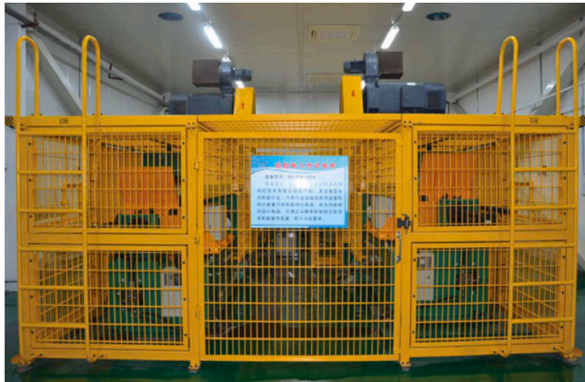
Fig. 7. Four-station durability testing machine.
