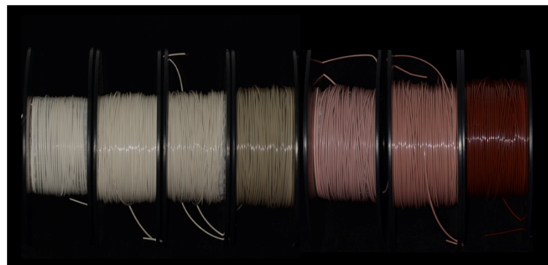
Figure 6. A series of dual-color PEEK filaments. From left to right: PEEK filaments with tooth-like colors (PEEK D1, D2, D3), pure PEEK filaments for contrast, and PEEK filaments with gingiva-like colors (PEEK G1, G2, G3).
