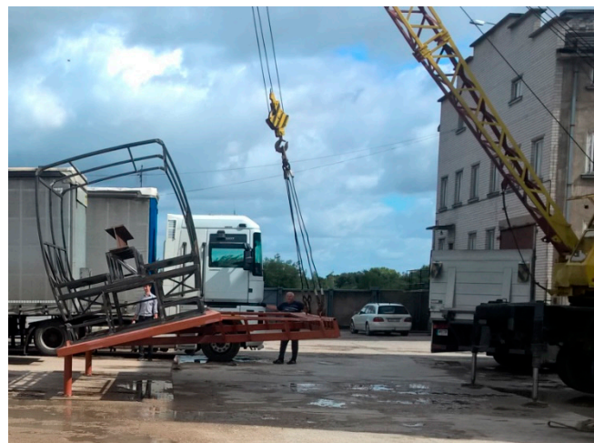
Figure 11. The safety frame before the natural rollover experiment.
