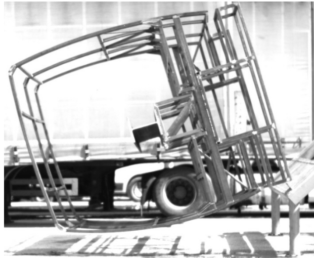
Figure 12. The safety frame 0.24 s after the beginning of the impact.
