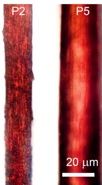
Figure 17. Images of the fibers obtained from PANI-O solutions P2 and P5, coagulated by three-component composition.
