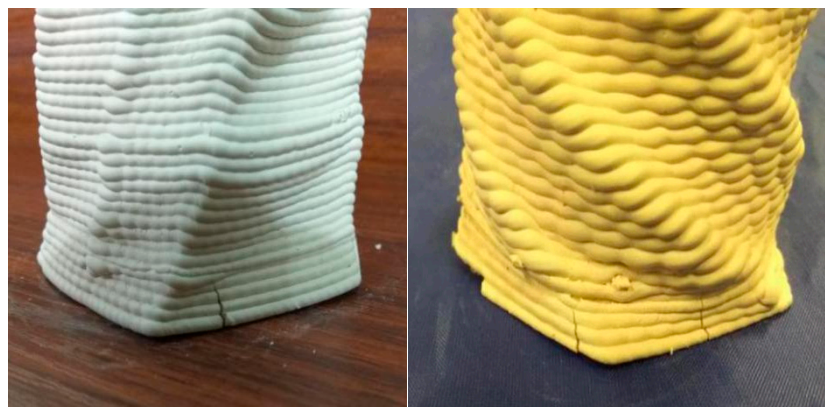
Figure 6. Cracks due to nonuniform drying.
