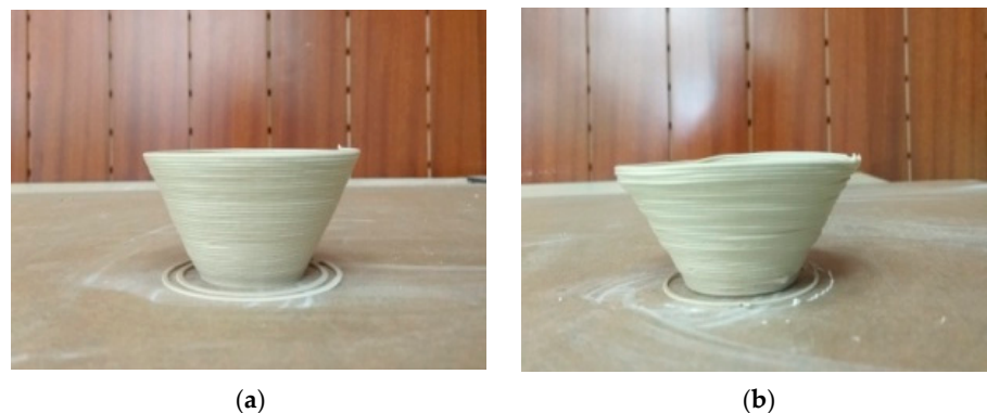
Figure 11. Conical thin-walled benchmark parts with in situ hot air flow drying: (a) cone angle as 30^\circ and (b) cone angle as 35^\circ .
