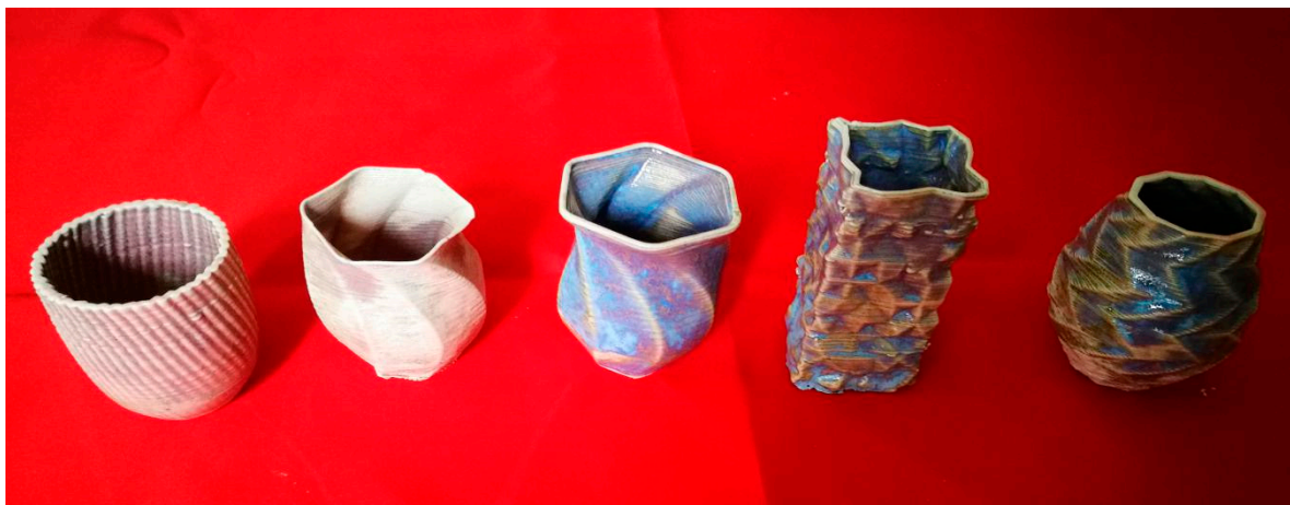
Figure 15. Sintered three-dimensional printed ceramic samples.
