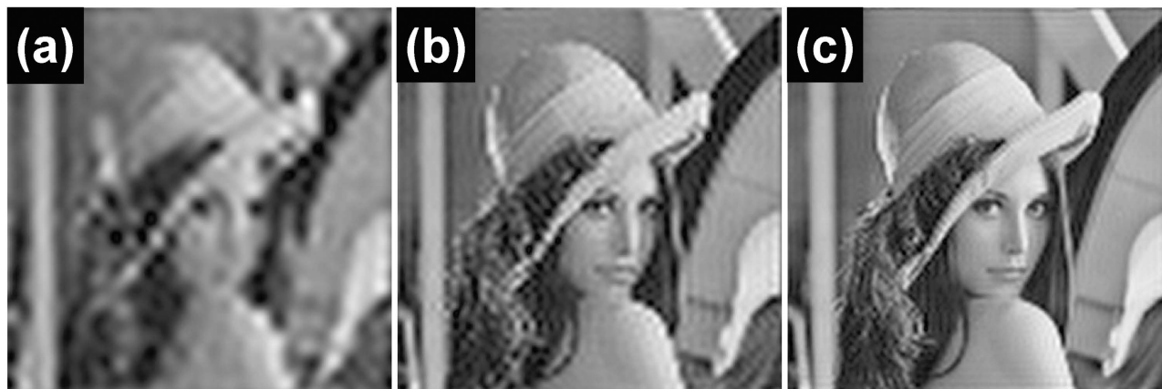
Figure 4. The image acquired by S-SLM with sampling parameters: (a) \Lambda = 80 nm and w = 40 nm, (b) \Lambda = 40 nm and w = 20 nm, and (c) \Lambda = 25 nm and w = 20 nm.
