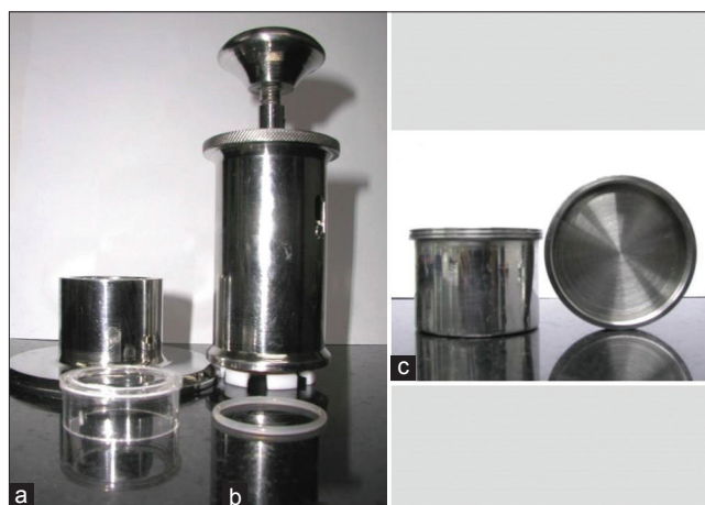
Figure 1. (a and b) Indigenously designed and patented mounting device for mounting human amniotic membrane onto a millicell insert, (c) In-house designed and patented stainless steel transport container for transportation of the graft to hospital site.
