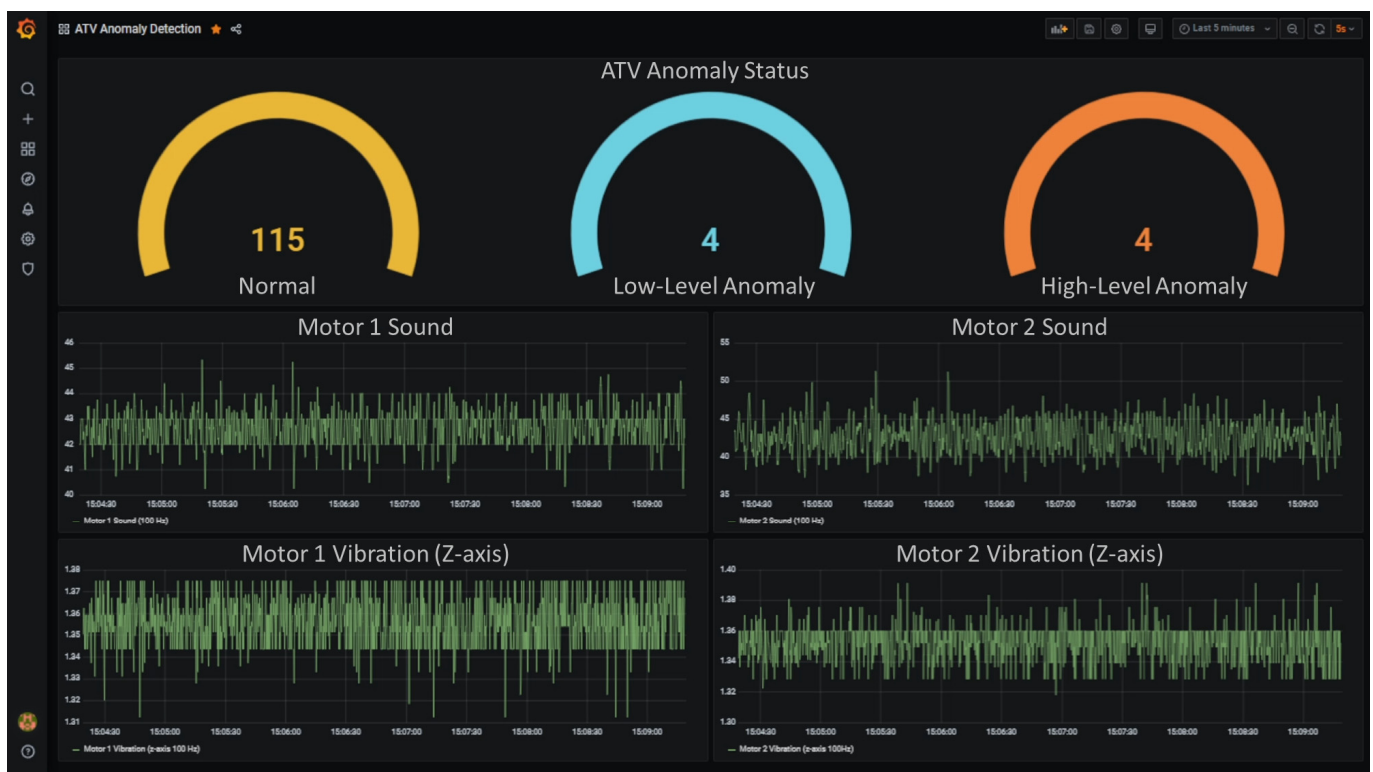
Figure 6. Grafana dashboards for real-time condition monitoring.
