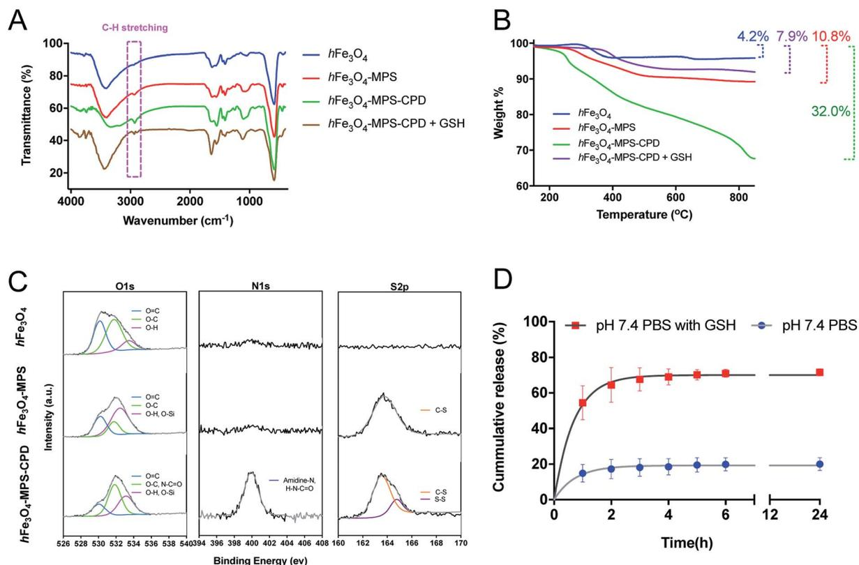
Fig. 2 (A) FT-IR spectra and (B) TGA decomposition curves for  $h\text{Fe}_3\text{O}_4$ ,  $h\text{Fe}_3\text{O}_4$ -MPS and  $h\text{Fe}_3\text{O}_4$ -MPS-CPD before/after GSH treatment. (C) XPS spectra for O 1s, N 1s and S 2p of  $h\text{Fe}_3\text{O}_4$ ,  $h\text{Fe}_3\text{O}_4$ -MPS and  $h\text{Fe}_3\text{O}_4$ -MPS-CPD. (D) Release profiles of cisplatin- $h\text{Fe}_3\text{O}_4$ -MPS-CPD in pH 7.4 PBS buffer with and without 10 mM GSH at predetermined time intervals over 24 h.
