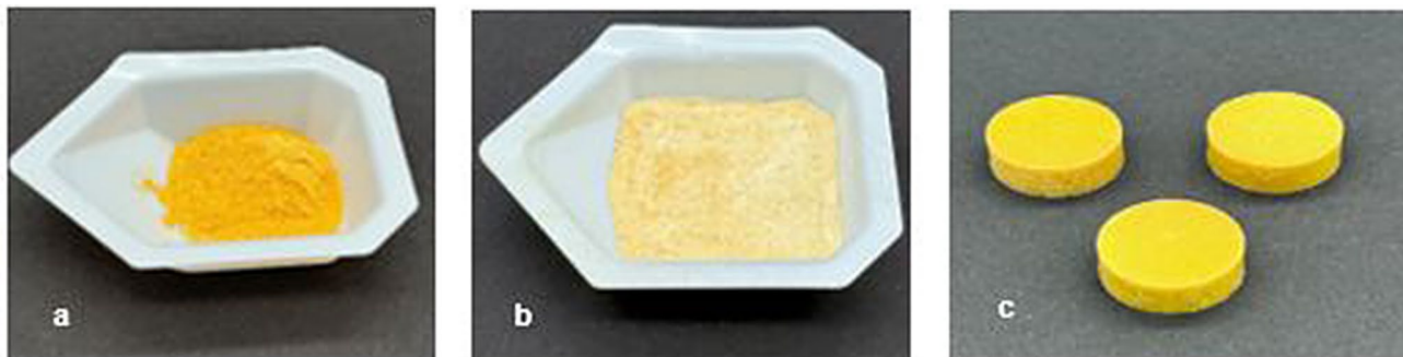
Fig. 2 Different formulations and appearances of AmBisome® (a) AmBisome® as pure powder; (b) AmBisome® powder mixed in PMMA powder; (c) hardened AmBisome® containing Copal specimens
