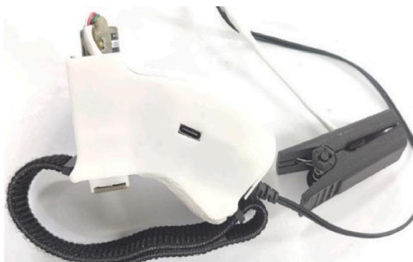
Fig. 1. The wearable hardware component of ZY-I type pulse diagnostic device.
