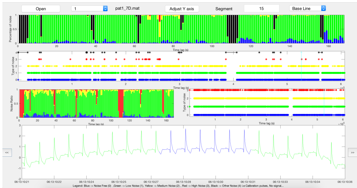
Figure 9. Noise maps' interface of the 7 day Holter recording (lead 1). See text for details.
