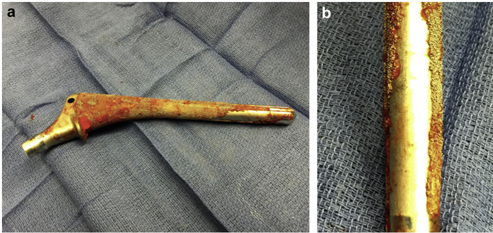
Figure 6. (a) Explanted femoral component with visible bead loss at the distal portion of the stem. (b) Close-up of the distal medial phase of the explanted femoral stem with bead loss.
