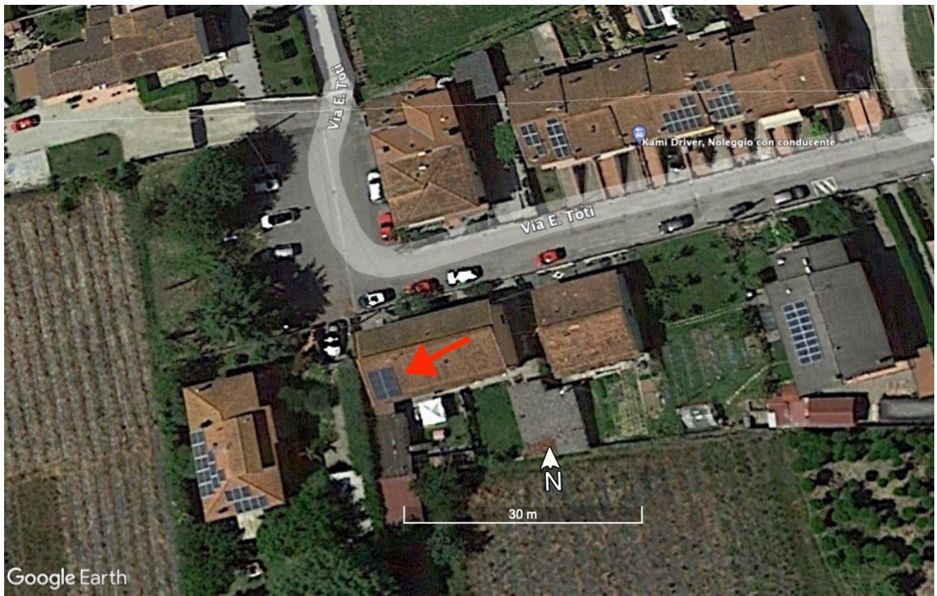
Figure 2. The red arrow indicates the photovoltaic modules (43.51° N, 10.48° E, 20 m a.s.l.) used in this study. The panel azimuth angle is 163° azimuth and it is tilted by 30° degrees. Image: Google Earth Pro (7.3.3.7786, 4 June 2021).
