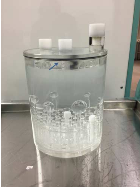
The mini-Jaszczak phantom (including both spheres and rods) Leakage of phantom shown by arrow.
