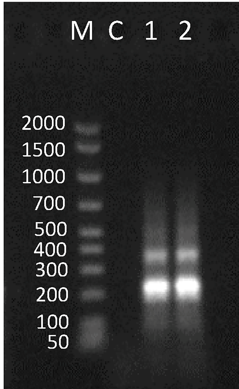
Fig 11. Assessment of CvA transcription. Agarose gel electrophoresis of CvA PCR performed on cDNA synthesized from RNA extracted from muscle and gonads of A. colbecki . M: marker; C: negative control; 1: A. colbecki muscle; 2: A. colbecki gonad.
