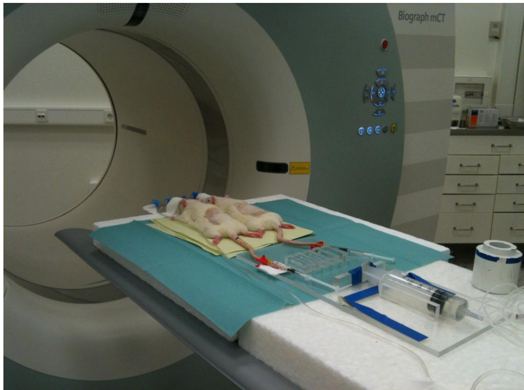
Figure 2 Experimental setting. Our experimental setting demonstrating two rats prior to positioning in the PET-CT scanner and homemade injector (two animals can be examined in parallel per scanning).
