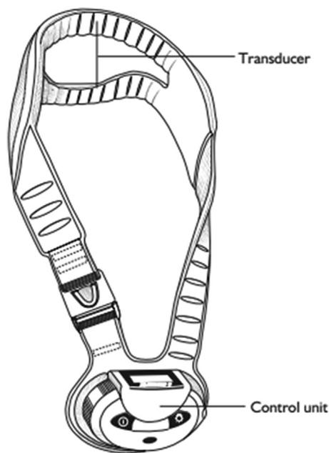
**Figure 4** Cervical-Stim pulsed electromagnetic field (PEMF) device.
