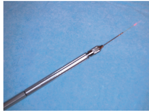
FIGURE 1: The optical fiber tips of 0.320 mm diameter (Nd:YAG laser—CTL-1503, Lasereinstruments, Warsaw, Poland).
