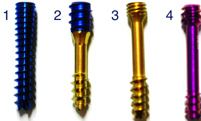
Fig 1. Competing screws. 1—Acumed Acutrak 2 Mini (AA), 2—Stryker TwinFix (ST), 3—Synthes 3.0 HCS with a long thread (SH), 4—KLS Martin HBS 2 Midi (MH).
