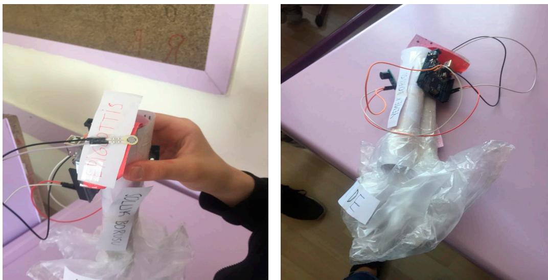
Figure 2. Epiglottis model with a thin film pressure sensor.
