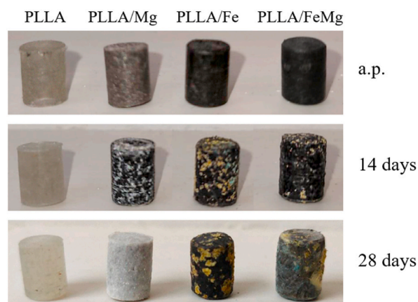
Fig. 2. Photographs of the cylinders (6 mm diameter, 9 mm height) in their as-processed and degraded states after 14 and 28 days of immersion in PBS. From left to right: PLLA, PLLA/Mg, PLLA/Fe and PLLA/FeMg.
