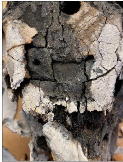
Figure 5. Post-processing reconstruction showing fragment association retaining depressed impact area.
