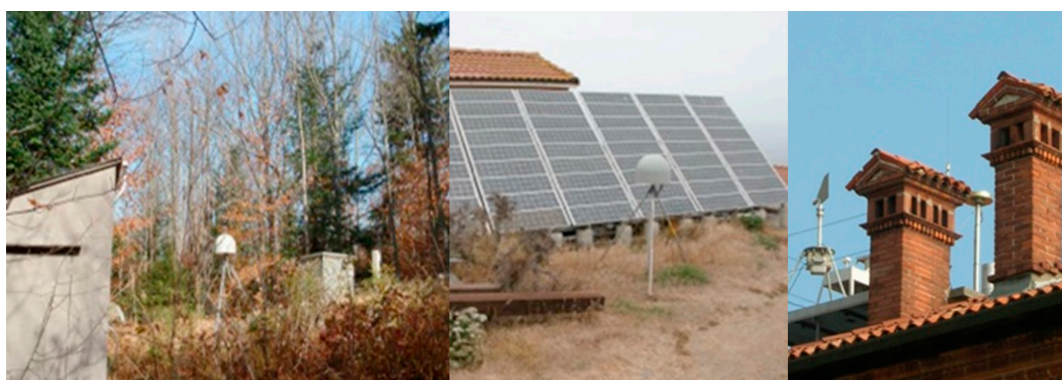
Figure 1. Examples of Poorly Sited CORS stations [15].
