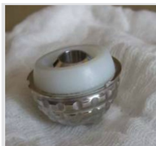
Figure 6: Picture showing the extracted dual mobility socket; note the absence of cement-implant bonding.
