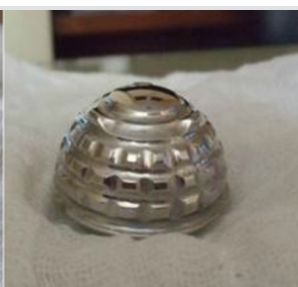
Figure 6: Picture showing the extracted dual mobility socket; note the absence of cement-implant bonding.
