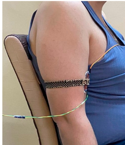
Figure 9. Acquiring the signal from the bicep muscle at relaxed state.
