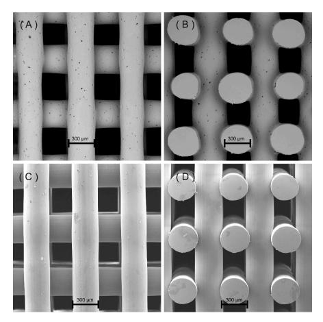
**Figure 2.** (**A**) Top view of a polycaprolactone (PCL) scaffold, (**B**) cross-section view of a PCL scaffold, (**C**) top view of a Polyethylene terephthalate glycol modified (PETG) scaffold, (**D**) cross-section view of a Polyethylene terephthalate glycol modified (PETG) scaffold. All scaffolds were designed considering a pore size of 350 μm.
