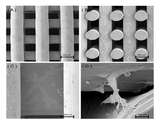
**Figure 7.** Cells on PETG-350 scaffolds after 14 days of cell seeding. (**A**) Top view image of the PETG scaffold, (**B**) cross-section image of PETG scaffold, (**C**) magnified image showing cells covering the PETG filament, (**D**) cells bridging adjacent layers.
