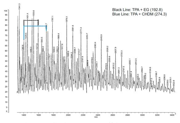
**Figure 1.** The Matrix-assisted laser desorption/ionization time-of-flight mass spectrometry (MALDI-TOF MS) spectrum of Polyethylene terephthalate glycol modified (PETG). Its characteristic repeated units are highlighted: 192.8 g/mol for the Terephthalic acid + Ethylene Glycol (TPA + EG) unit and 274.3 g/mol for Terephthalic acid + Cyclohexanedimethanol (TPA + CHDM).
