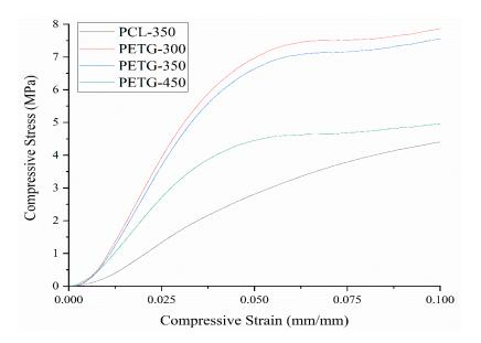
Figure 3. Stress vs. strain curves for PCL scaffolds and PETG scaffolds with different pore sizes.
