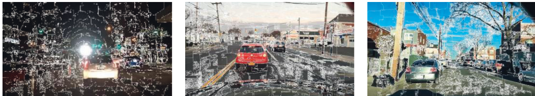
FIGURE 2: Example of superpixel image segmentation by means of SLIC.
