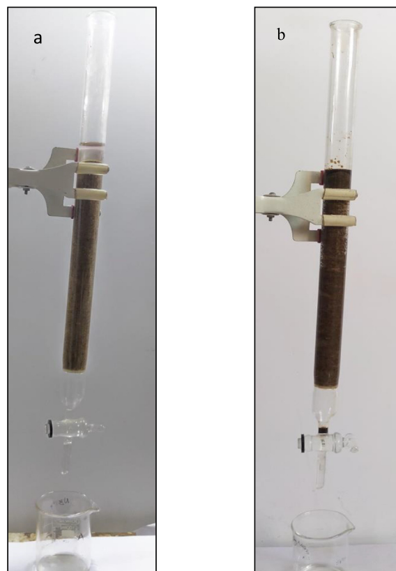
Fig. 2. Sand pack column. (a) Before oil incubation, (b) After oil incubation.
