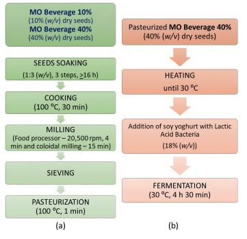
Figure 1. (a) *M. oleifera* beverage and (b) yoghurt-like manufacturing procedures.
