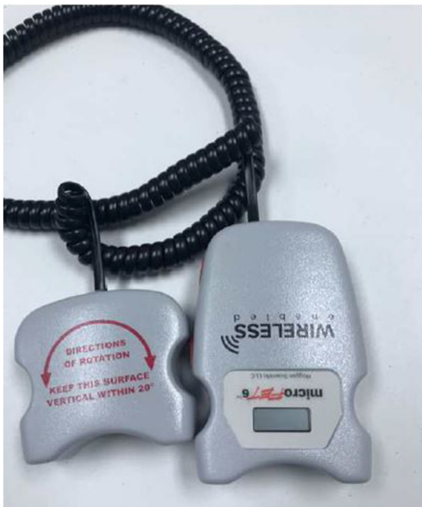
Figure 1: Electronic goniometer to measure neck range of motion.
