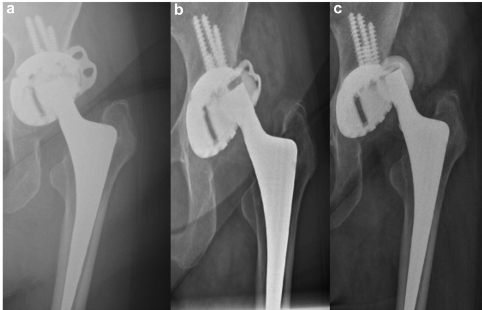
Figure 1. Radiographs from April 2019 (a), November 2020 (b), and January 2021 (c) showing the progression of the massive polyethylene and metal wear leading to penetration of the ceramic head through the superolateral part of the cementless titanium cup. The bubble sign of severe metallosis can be seen in Figure 1c.
