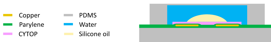
Figure 3. Cross-section of a schematic of a single, fully assembled electrowetting cell. The well for containing the liquids for electrowetting was affixed using PDMS, and a silicone oil droplet was placed over the hydrophobic region of the flexible dielectric surface defined by the patterned CYTOP before being surrounded by water and sealed into the well.
