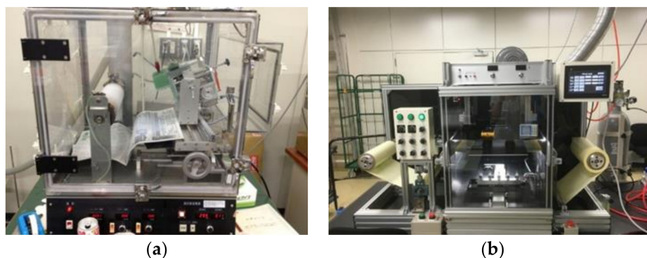
Figure 2. The lab scale electrospinning set-up (a) and pilot scale electrospinning set-up (b).
