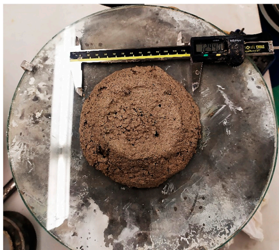
Figure 3. Image of a lime mortar representative slump obtained in agreement with EN 1015-3.
