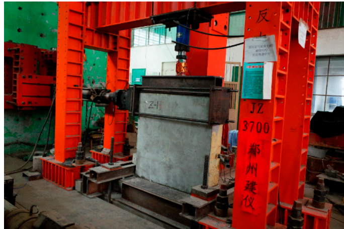
Figure 2. Scene photos of test devices and wall specimen.
