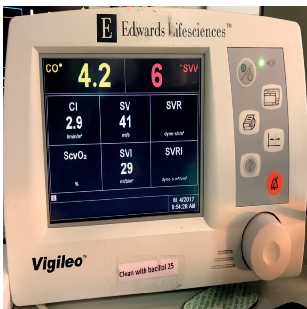
Fig. 1. FloTrac (Vigileo system, Edwards Lifesciences Inc) – non-invasive monitoring of cardiac output
