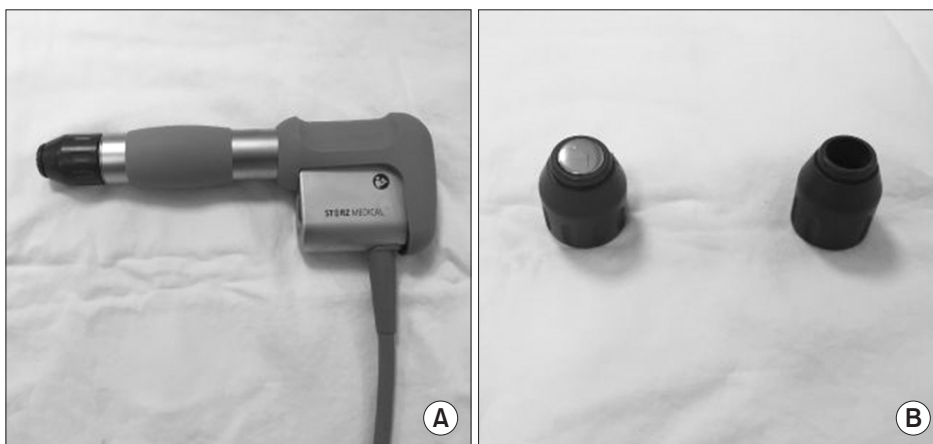
Fig. 1. (A) The stimulator. (B) The stimulator head and transmitter, and the stimulator head without the transmitter. In the radial extracorporeal shock wave therapy group, stimulation was delivered by the stimulator head with the transmitter; however, in the control group, patients received the same frequency but that of air pressure via the stimulator head without the transmitter.
