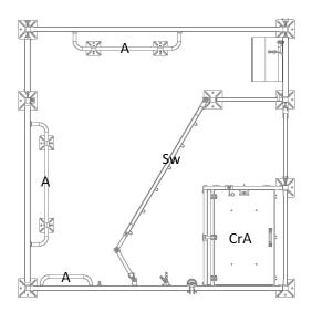
**Figure 2.** Single loose housing pen (LH). CrA = creep area, Sw = swing gate, A = anti-crushing bars. © Big Dutchman International GmbH, Vechta, Germany.
