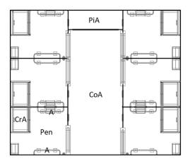
**Figure 3.** Group-housing system for lactating sows (GH). CrA = creep area, A = anti-crushing bar, CoA = common area, PiA = piglet area. © Big Dutchman International GmbH, Vechta, Germany.
