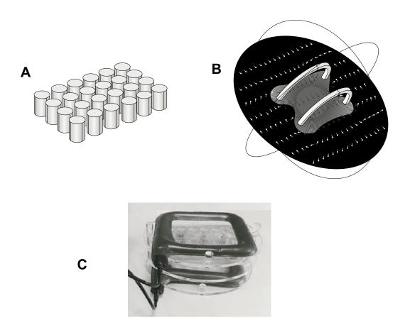
**Fig. (1).** Description of ELF MF exposure system. Panel A shows the schematic geometry of multiwells used in a simulation model. Panel B shows a computer modeling of the magnetic field between coils, with arrows indicating magnetic field (H) strength and direction, demonstrating a constant distribution within whole multiwell plate. Panel C shows a picture of the exposure system with the Plexiglass holder keeping multiwell plate between coils.
