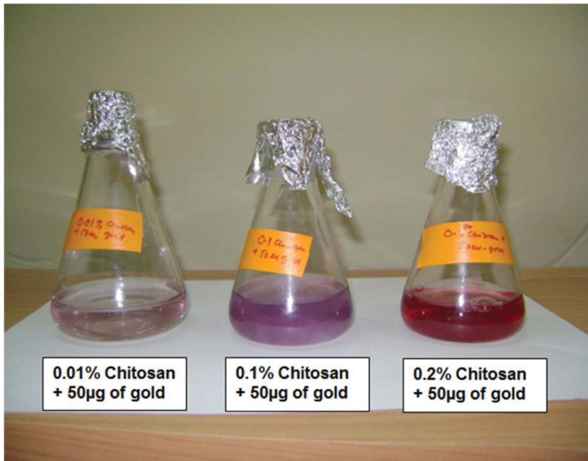
Figure 2. Formation of chitosan gold nanoparticles. Varying the ratio of gold salt to chitosan in the medium helps in achieving size controlled synthesis of nanoparticles. Nanoparticles formed in the last beaker were used for animal experimentation. doi:10.1371/journal.pone.0057094.g002
