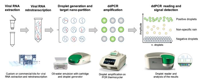
Figure 10. Schematic workflow of the ddPCR detection system. ddPCR, droplet digital PCR.
