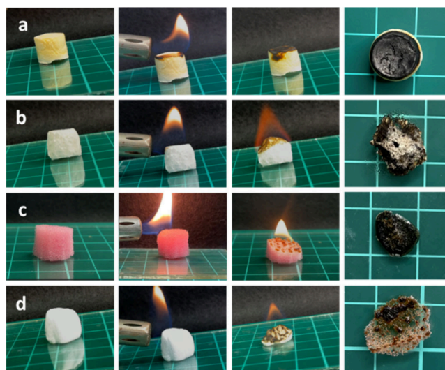
Figure 6. Photographs demonstrating the behavior under open flame of (a) CSNFs-DACMC (2.5 wt %, FT -25\text{ }^{\circ}\text{C} , TT 4\text{ }^{\circ}\text{C} ) and commercial (b) cellulose, (c) PU, and (d) PS foams.
