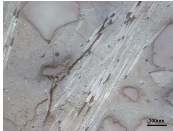
Figure 14. Matrix-fiber-aggregate connectivity against cracks in the composite structure. Sample M50-5.
