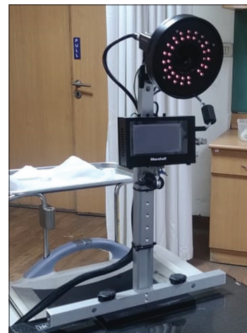
Figure 2: The IR camera captures and monitors infrared light, which is often reflected off markers placed on the patient's body. These markers help the system to track even subtle movements, which is essential for maintaining precision throughout the treatment
