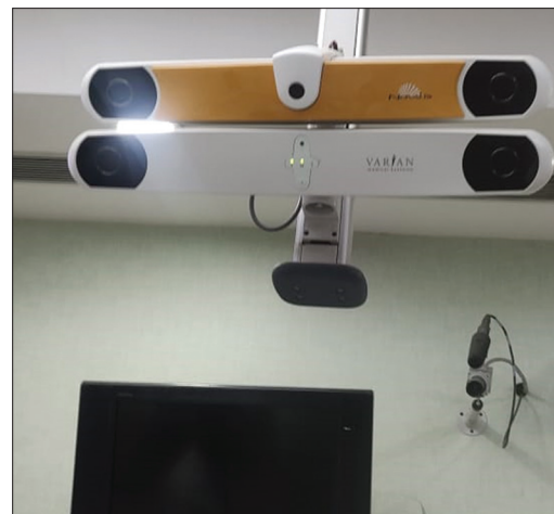
Figure 3: Real-time monitoring: During treatment, the system compares the patient's current position with the planned treatment position. If the patient moves out of the set threshold, the system alerts the clinicians or even pauses the radiation beam, preventing mistargeting
